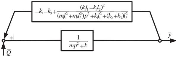
Fig. 3. Transformed structural scheme with the exception of the coordinate  $\bar{\varphi}$
