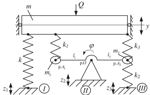
Fig. 1. The design scheme of a vibration protection system with an intermediate solid body (inertial lever of the second kind)
