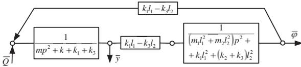
Fig. 2. Structural diagram of the vibration protection system with two degrees of freedom under force perturbation
