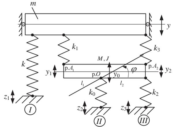
Fig. 4. Calculation scheme of a vibration protection system with an intermediate solid on an elastic support
