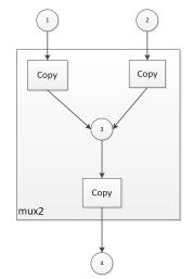
Fig. 5. A dataflow model of the multiplexer mux2
