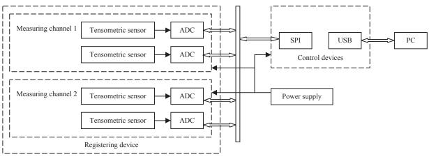
Fig. 1. Block diagram of the tensometric analyzer
