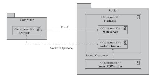
Fig. 2. Smart-M3 Control Panel system architecture
