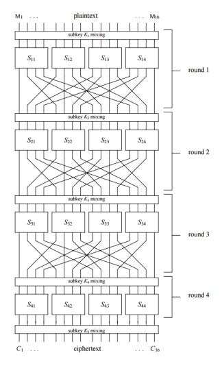
Fig. 1. Substitution-permutation block cipher with block length 16 and four rounds.
