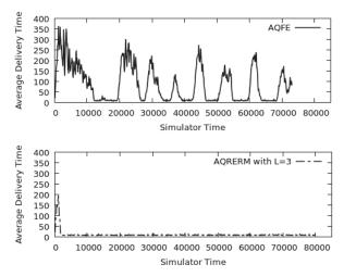
Fig. 11. Stability of routing under AQFE and AQRERM for  $\lambda = 3$
