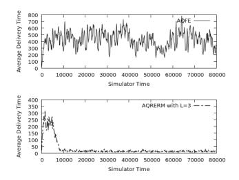
Fig. 12. Stability of routing under AQFE and AQRERM for  $\lambda = 3.5$
