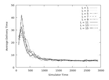
Fig. 6. Performance of AQRERM for various L under low load
