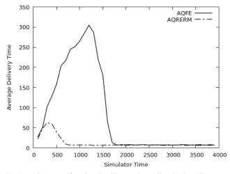
Fig. 10. Performance of routing algorithms under medium load conditons
