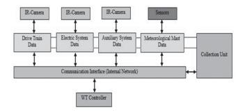
Fig. 2. Internal communication network architecture within WT
