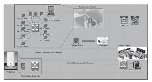
Fig. 4. OPNET based communication network model for monitoring WT using IR-camera
