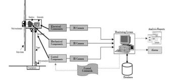
Fig. 1. Schematic diagram of IR-camera based wind turbine monitoring
