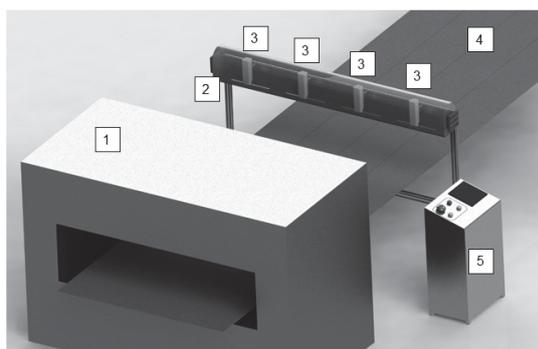
Fig. 2. Arrangement of the complex on the production line, where: 1 - slitting machine, 2 - bearing frame, 3 - cameras, 4 - corrugated board web with cuts, 5 - operator station
