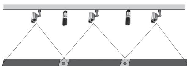
Fig. 3. The mounting of cameras and laser pointers on the frame
