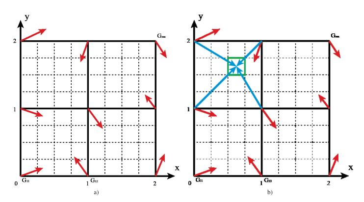
Fig. 2. Stages of Perlin's noise formation: a) Formation of a grid and normal vectors; b) Calculation of vectors from grid cell corners to the considered pixel direction
