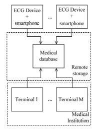
Fig. 1. Heart monitoring system scheme
