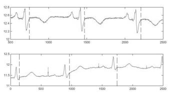
Fig. 6. J-point detection results: upper - normal ECG record; lower - ECG record with artifacts
