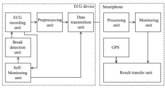
Fig. 2. ECG device scheme
