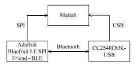
Fig. 10. Wireless protocol test scheme
