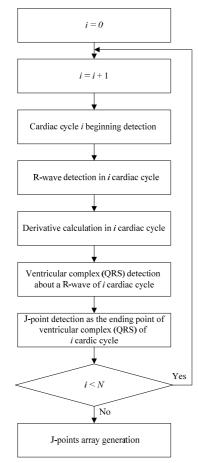
Fig 5. J-point detection algorithm scheme
