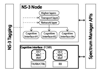
Fig. 1. FCMR Cognitive Interface block architecture considered at ns-3 implementation
