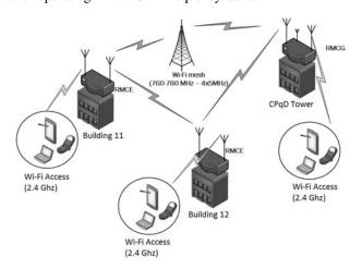
Fig. 2. Experimental network topology of CCMN installed at CPqD facilities
