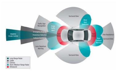
Fig. 1. A car equipped with ADAS (source: [2])
