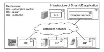
Fig. 5. Enhanced infrastructure for a Smart-M3 application
