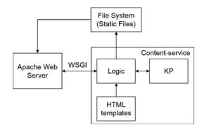
Fig. 3. Content-service architecture: the use of matured web technologies to improve the fault tolerance
