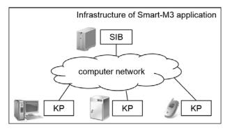
Fig. 1. Smart-M3 application infrastructure consists of the deployed SIB and service-responsible KPs
