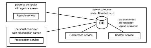
Fig. 2. Deployment options in the SmartRoom infrastructure: Conference-service and Content-service are near the SIB, Agenda-service and Presentation-service are near their multimedia screens
