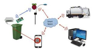
Fig. 1. Hardware components used in the smart waste system
