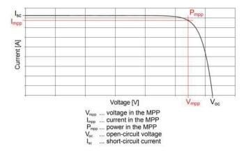
Fig. 3. Output power characteristics of a PV cell
