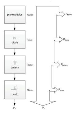
Fig. 9. Structure with power losses
