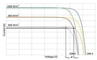
Fig. 4. I-V curve under different ambient conditions
