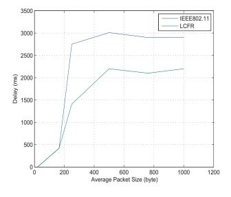
Fig. 5. Delay, 20 network nodes
