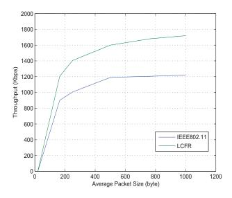
Fig. 3. Throughput, 50 network nodes
