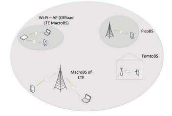
Fig. 1. Structure of heterogeneous network.
