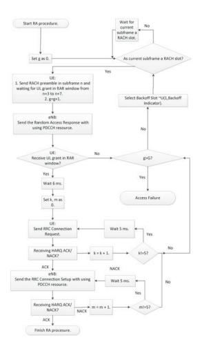
Fig. 5. Algorithm of RA procedure.
