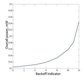
Fig. 6. Dependence of the overall power on the value of backoff indicator.
