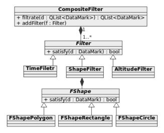
Fig. 4. Spatial filters class diagram
