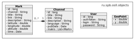
Fig. 7. Class diagram of ru.spb.osll.objects package
