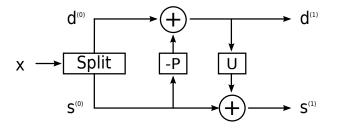
Fig. 1. Diagram of a lifting step
